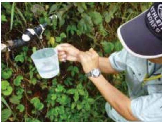
Photo 2.16: Direct measure of Leakage Volume
