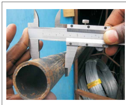
Photo 5.9: Measuring pipe diameter
