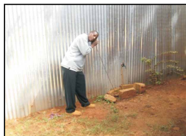
Photo 2.11: Leak detection using Listening Stick
