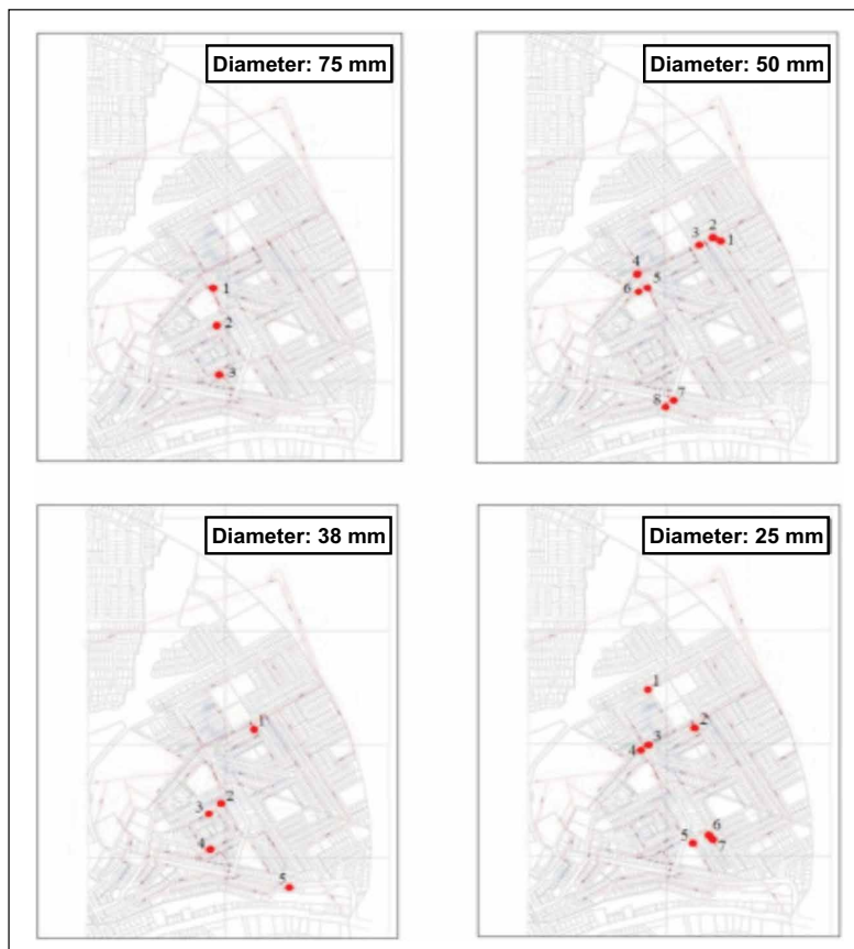
Figure 2.5 Location of Replaced and Newly Installed Gate Valve
