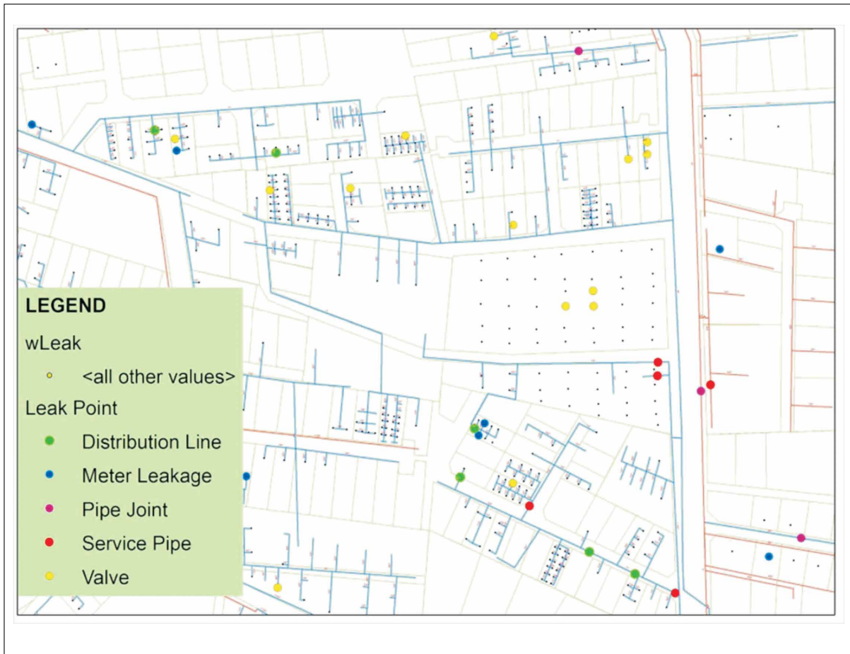
Figure 3.5 Leak survey map on GIS (EWASCO)
