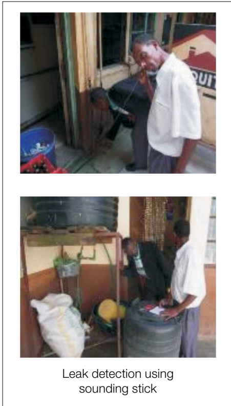
Photo 3.3 Leak detection activity
