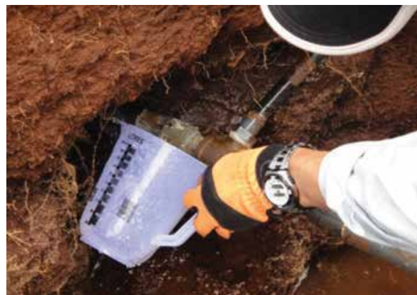
Photo 2.16: Direct measure of Leakage Volume
