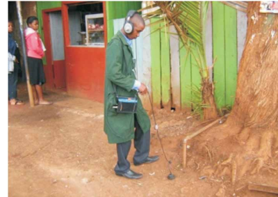
Photo 2.15: Leak detection using Electronic leak detector
