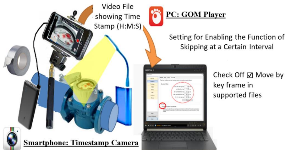
Figure 13.5: Measurement of Hourly Water Flow with Smartphone and Free Software
