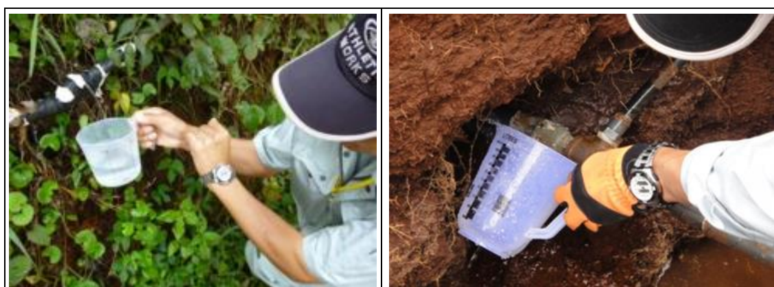
Figure 8.4: Measurement at Actual Leakage Point
