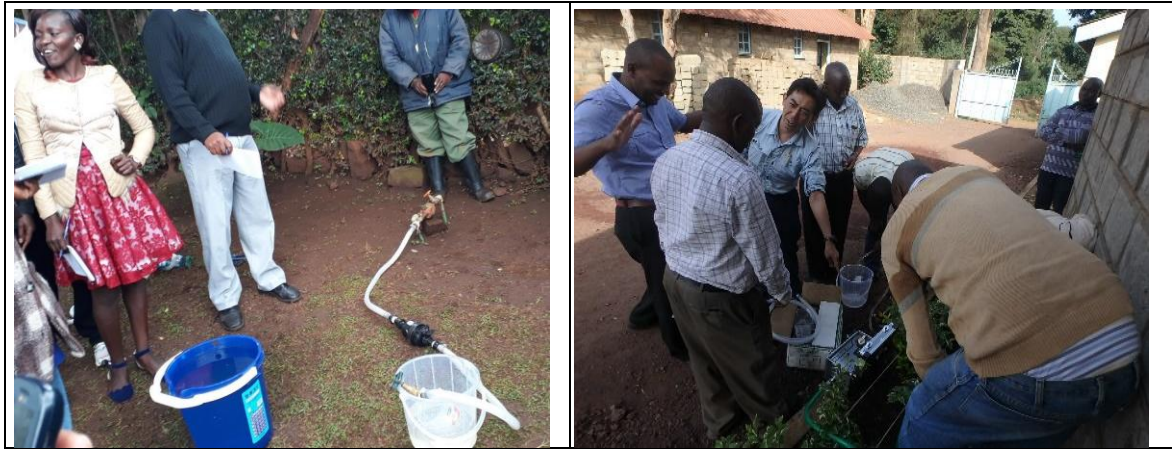
Figure 6.4: Meter Testing using Portable Test-meter and Calibrated bucket
