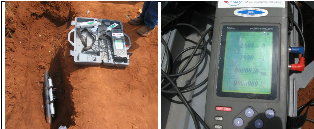
Fig. 5.30: Flow Measurement Using UFM
