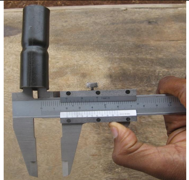
Fig. 2.2: Measuring inside diameters of uPVC repair coupling with vernier caliper
