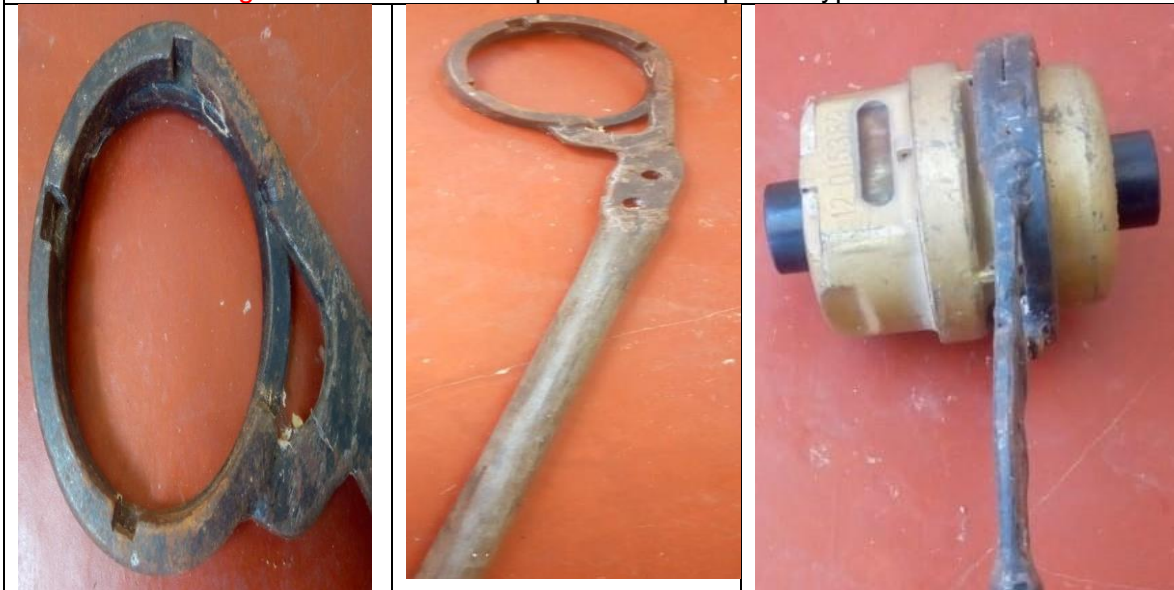
Fig. 8.2: Custom-made spanner for Volumetric Type Meters
