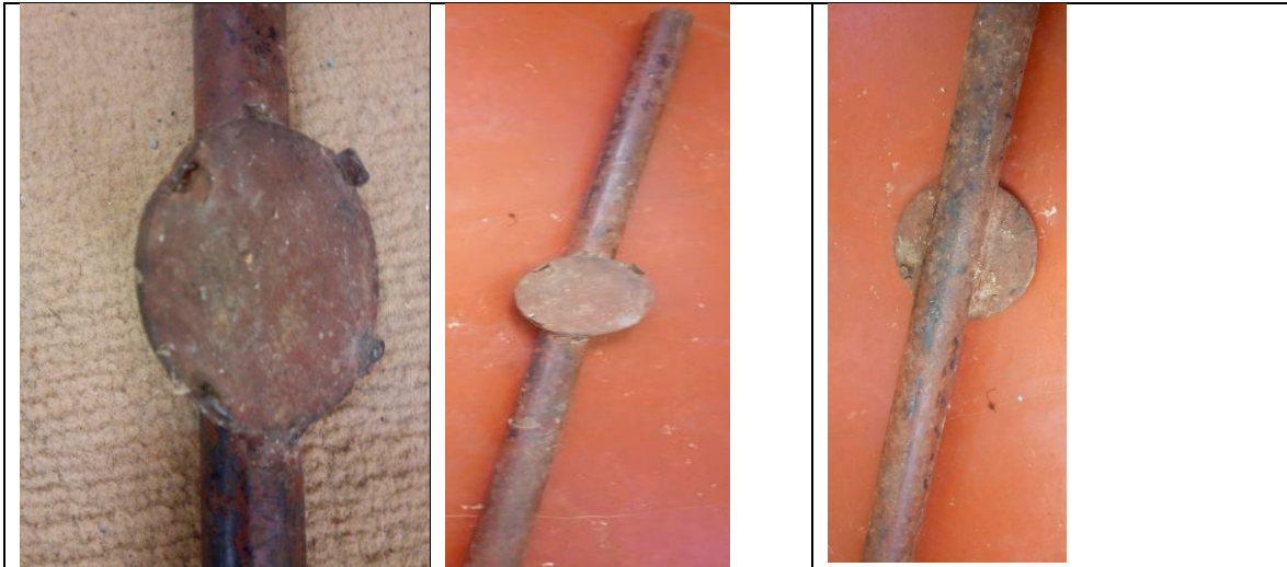
Fig. 8.1: Custom-made spanner for Propeller Type Meters
