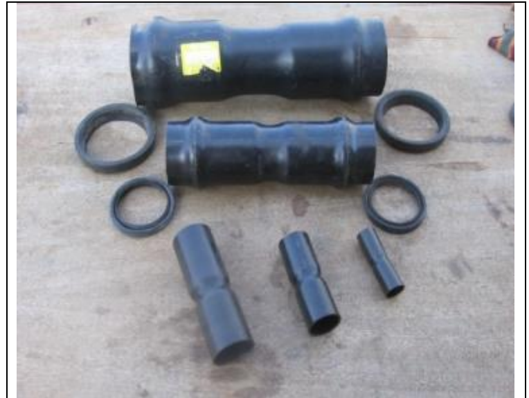
Fig. 2.4: Rubber ring couplings (dia \geq 63\text{mm} ) and Bonding Joint Couplings (dia < 63\text{mm} )
