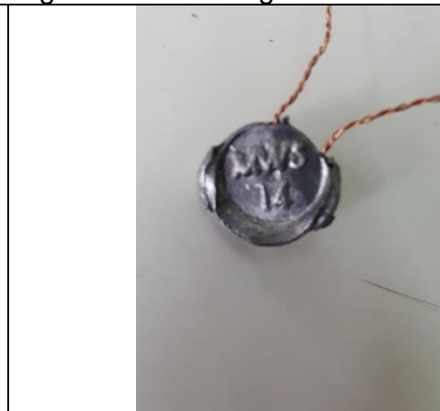
Fig. 8.10: Sealing lead stamped by Pliers No. MWS14
