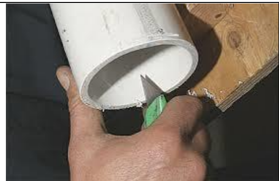
Fig. 2.7: Unchamfered dimensions being deburred
