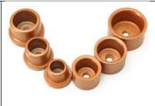
Fig. 2.28: Male & female fusion sockets (die pairs)
