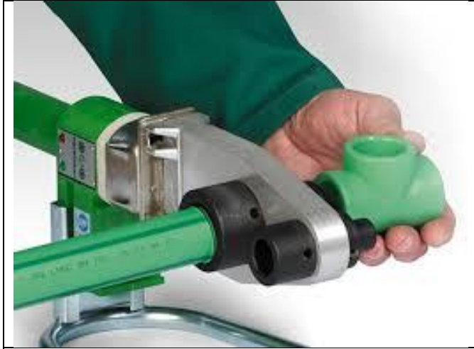
Fig. 2.29: Heating PPR pipe & tee socket
