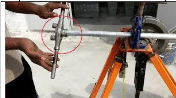
Fig. 2.31: Threading of pie with diestock
