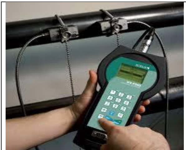
Fig. 5.15: Side-mounted sensors on PVC pipe
