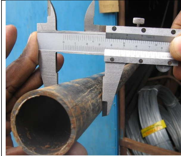
Fig. 2.1: Measuring outside diameters of uPVC pipe with vernier caliper
