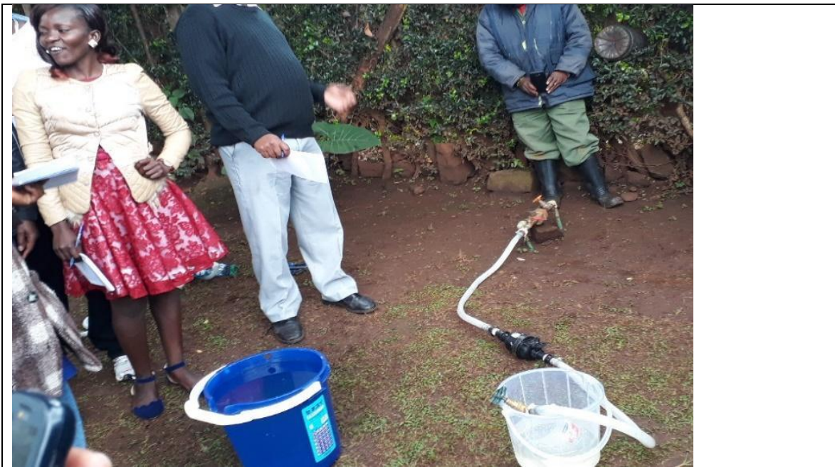
Fig. 8.4: Testing a meter using calibrated bucket and a portable test meter
