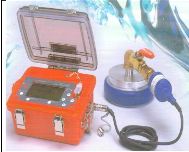
Fig. 6.9: Self-recording water pressure measuring device model
