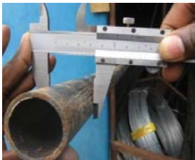
Figure 8.11: Checking Pipe diameter Internal and External using vernier calliper
