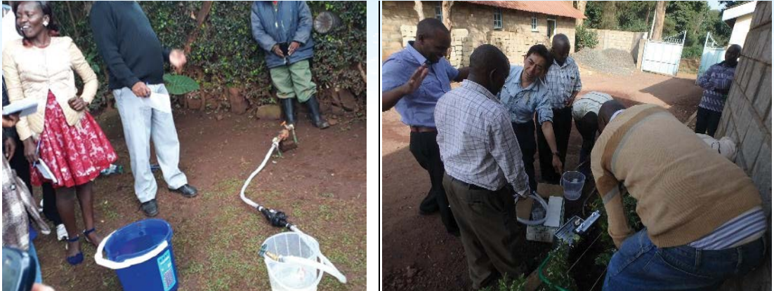
Figure 6.4: Meter Testing using Portable Test-meter and Calibrated bucket
