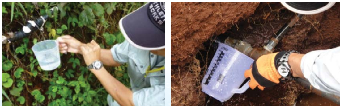
Figure 8.4: Measurement at Actual Leakage Point
