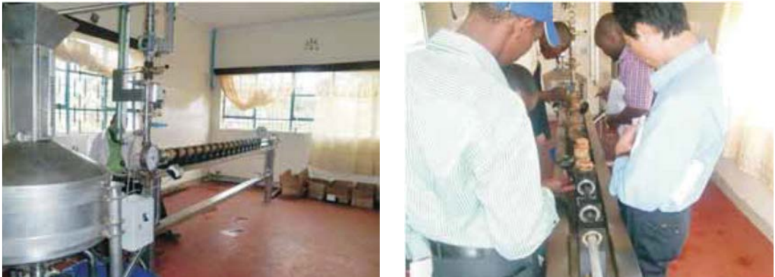
Figure 7.5: Water meter test bench
